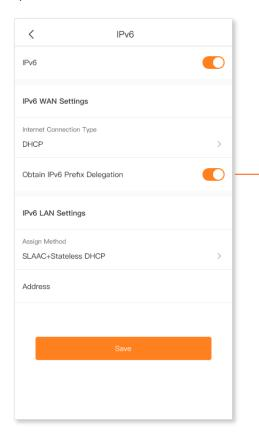
When the option is enabled, the LAN port of nova obtains IPv6 prefix from its upstream device.
